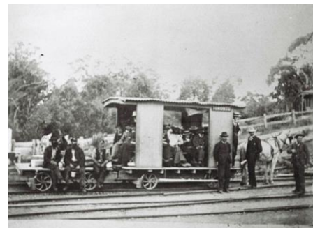
A rough horse-drawn tram with trolley trailer working the private Toronto Branch Line. The Line was later converted to Government-run heavy rail. Source: Lake Macquarie Library.
